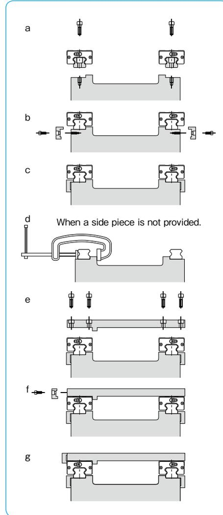
**When Reference Surface is Not Provided on Adjustable Side**
