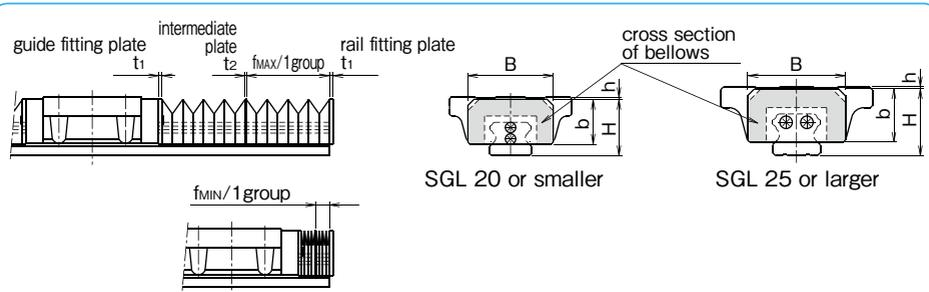
Note: Please do not unfasten the guide fitting plate screws. The slide guide becomes unfunctional if the guide fitting plate is removed.
