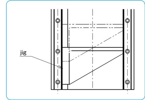
Figure A-18 Using Base Reference Surface
