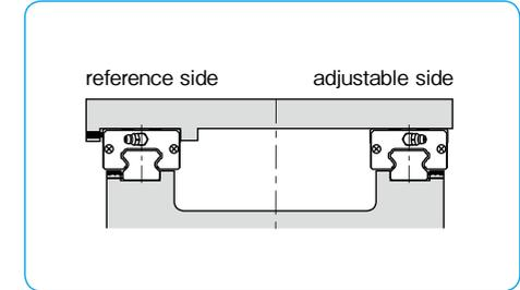
Figure A-10 Using Side Plate
