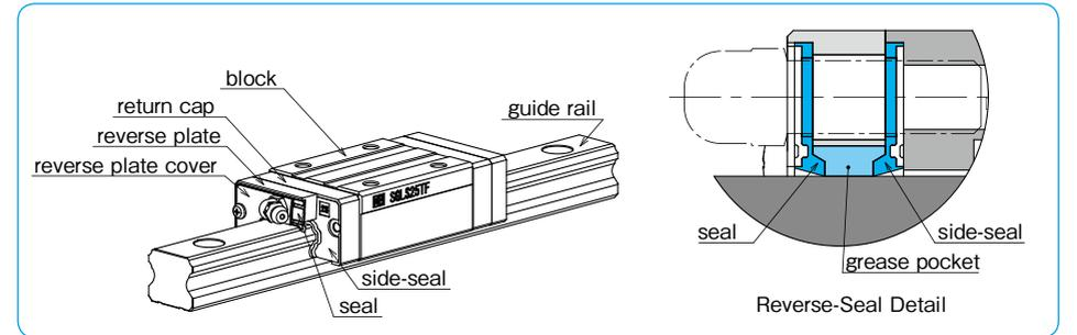
Reducing Grease Leakage
