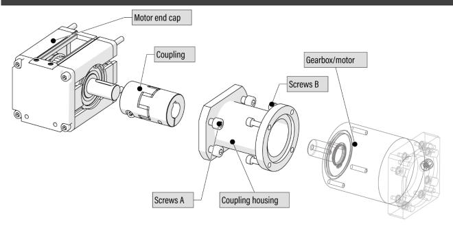
1. Insert the actuator side hub onto the shaft, the shaft end should coincide with the inner face of the hub, tighten the hub screw with the correct torque.
