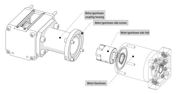
3. Insert the motor/gearbox into the bell housing by first matching the coupling and then the mounting holes, fasten with screws B and tension to the proper torque.
