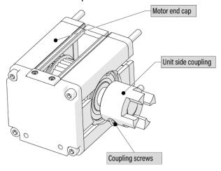
2. Connect the flange to the actuator (right or left side as needed) with the 4 screws A
